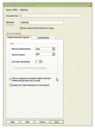
Wireless Protected Access (WPA) is the new standard in the wireless security. However, not all wireless cards and adapters support this technology. Please check your wireless adapter's user manual to check if it supports WPA. Instead of a hex key, WPA uses only passphrases, which are much easier to remember.
